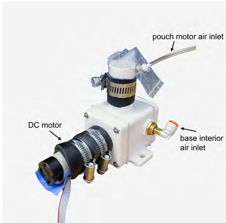
Figure 5.2: Fabricated single-base assembly for the pneumatic manipulator. The annotated diagram highlights the critical hardware integration points, including the pressure inlets for the chamber and the DC motor that guides the vine robot material. This rigid interface ensures no pressure is lost during the deployment of the robot into the workspace.
